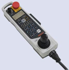
Joystick-box V2 with speed adjustment knob, standard accessory.
